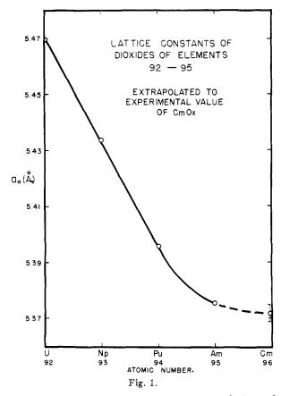
lattice constants. A reasonable extrapolation of the smooth curve would give  $\sim 5.37$  for the expected value of CmO<sub>2</sub>. Our value of 5.372 would indicate that the ratio of O/Cm must be close to 2, showing the existence of an "average valence" of Cm approaching 4.
